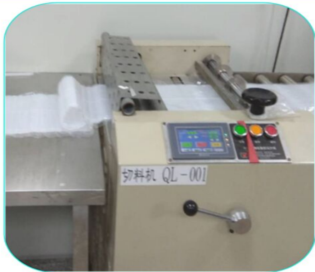
Automatic Cutting After Rubber Mixing
