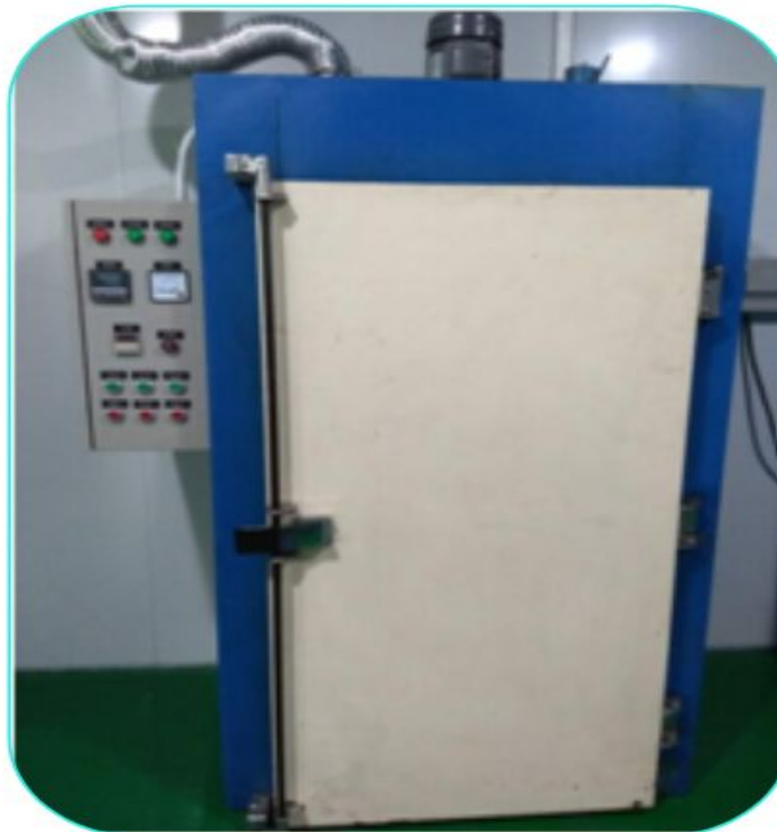
Constant-temperature Drying Oven - Product Drying
